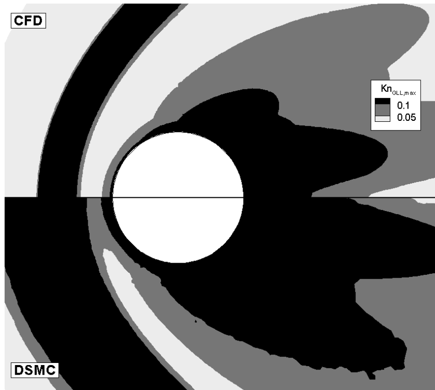
Figure 13: Kn around cylinder in Mach 10 argon: Re_\infty = 289 [54]
