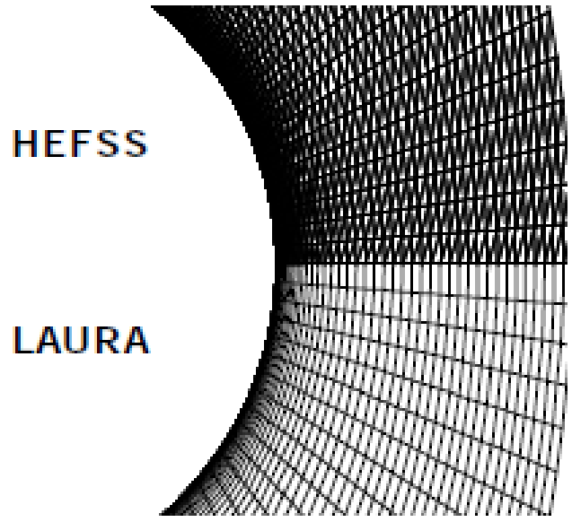
Figure 2: Structured grid (bottom) and equivalent uniformly biased unstructured grid (above) in Ref. [32]
